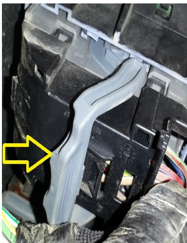
4. Pull back on the lever and remove the connector.
