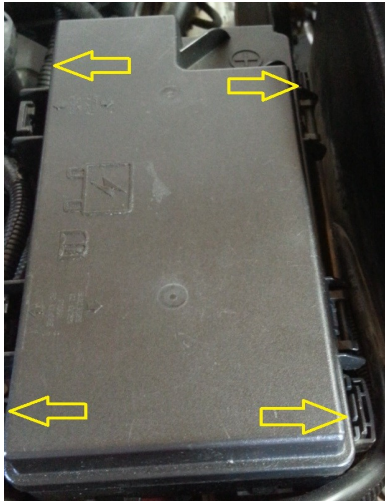
1. Lift up the TIPM by unlatching the 4 retaining clips, to gain access to the bottom connectors.
